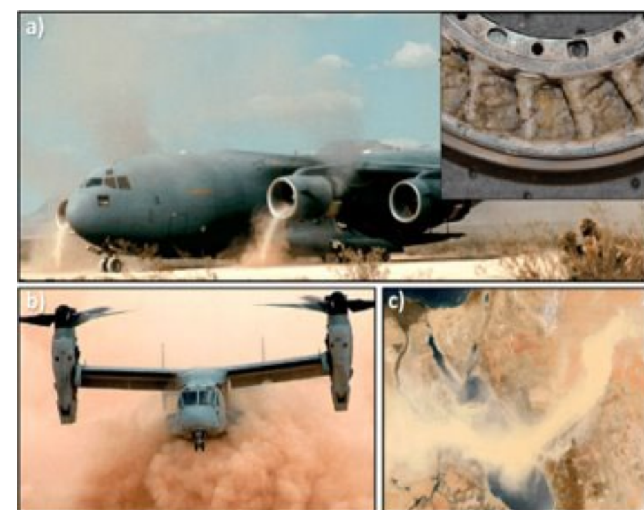
Figure 1: Example of CMAS entering turbine engines.
